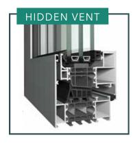
For a modern minimalistic appearance MasterLine 8 offers the Hidden Vent system. With Hidden Vent profiles the vents are covered by the outer frames and transoms, which allows for a concealed install of the opening elements behind the window reveal.
